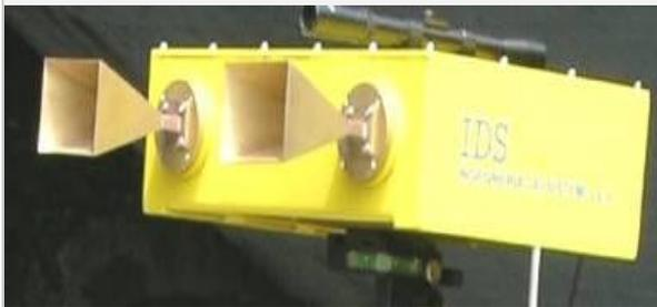
**Ground-based synthetic aperture radar (GB-SAR)**
