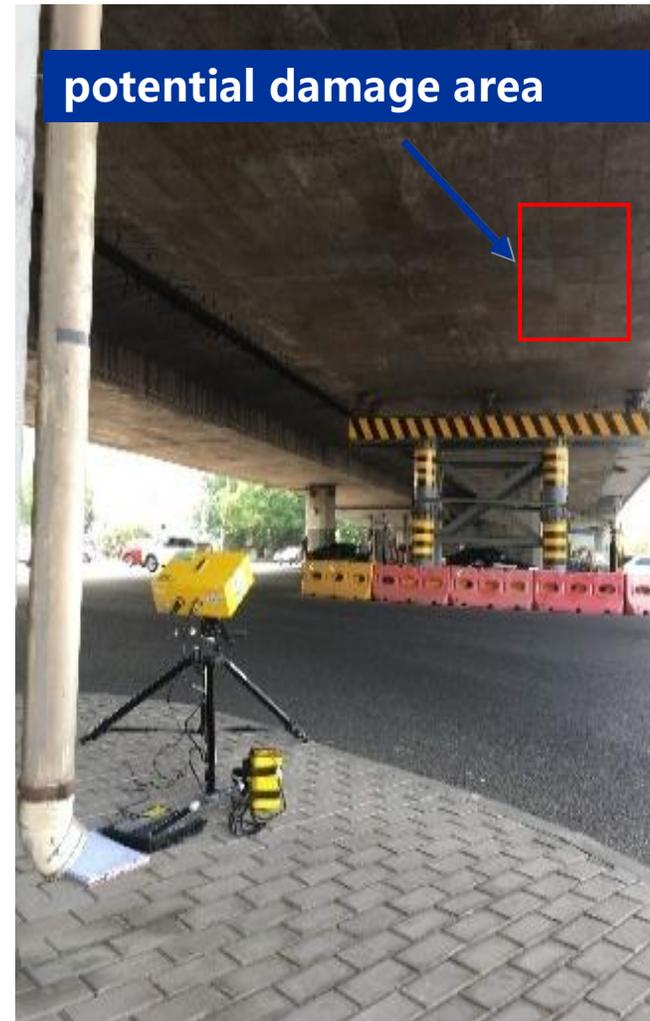
Calculating **point cloud curvature** can accurately reflect potential damage to the undersurface of bridges
