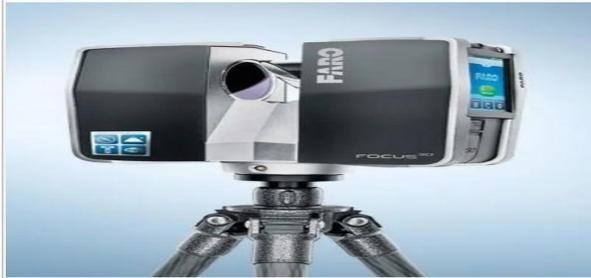
**Terrestrial Laser Scanning (TLS)**
